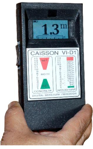
A reliable instrument for moisture testing in materials such as concrete, timber, stone, plastic, fiber glass etc. An indispensable tool for construction industry professionals to test before continuing the construction process. The **V1-D1** is pinless and does not damage the substrate under test.
